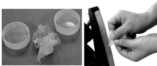
**5.4** Please apply the grease shown in the picture to the smooth surface of side bearings.
