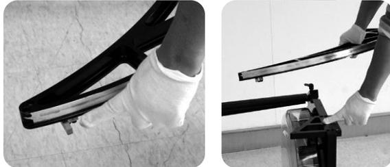
**5.2** Mount the left side bearing as shown in the picture, then secured it with 5pcs M6x25mm Allen screws, as shown in pictures.
