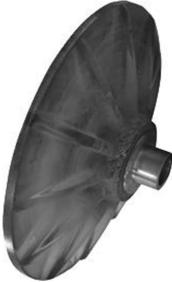
Instead of a heavy mirror blank at the standard 1:6 thickness ratios (1 cm thick for every 6 cm in diameter - so they won't flex and sag out of shape under their own weight), the StarGate 18 uses a thin composite mirror with sagittal reinforcements. This specific construction retains the same sturdiness as a standard 1:6 thickness ratio but is far less massive and will reach rapidly thermal equilibrium. The secondary flat mirror uses a cellular structure for the same purposes.
