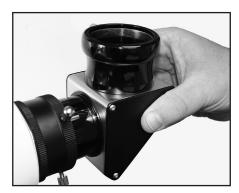
Tighten the set screw on the adapter ring to hold the diagonal in place.
