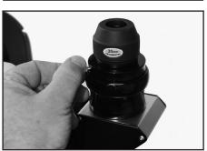
To remove the eyepiece, loosen the set screw on the diagonal and slide the eyepiece out.
