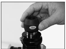
3. Tighten the set screw on the star diagonal to hold the eyepiece in place.
