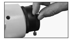
2. Slide the 2" barrel end of the diagonal into the focuser adapter ring.
