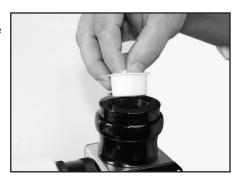
2. Slide the chrome portion of the eyepiece into the diagonal.
