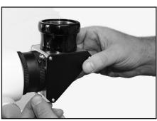
If you wish to change the orientation of the diagonal, loosen the thumb screw on the focuser draw tube. This will allow the diagonal (or camera for photography) to rotate freely. Rotate the diagonal to the desired position and tighten the screw.
