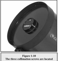
he three collimation screws are located on the front of the secondary mirror housing.
