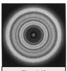
**Figure1-12** A collimated telescope should appear symmetrical with the central obstruction centered in the star's diffraction pattern.
